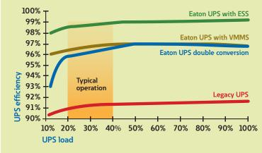
Efficiency generally dips as load levels decrease. However, ESS technology operates at 99 percent efficiency even at low-load levels, providing you with real energy savings. "ESS is a great system, and it's one of the main reasons we decided to go with this solution. If we are going to keep these units for 10-plus years, a few percentage points in efficiency really add up . . . [They] allow me to be more competitive in terms of being able to sell colocation."
